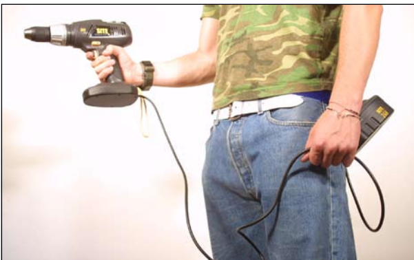
Figure 5. Cordless drill – reducing weight (working prototype)
